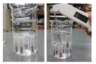
individual tube rises, take the temperature of the surrounding liquid and mark it on the tube with a colored pencil.
